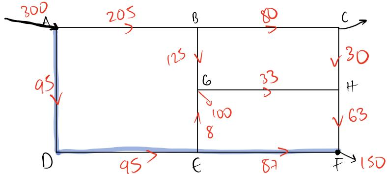
$$\begin{aligned} P_F &= P_A - \Delta P_{AD} - \Delta P_{DE} - \Delta P_{FF} & \Delta P = h_f \cdot \gamma \\ &= 489,5 - 9,79 \cdot 3,82 - 9,79 \cdot 14,7 - 9,79 \cdot 14,4 \end{aligned}$$
