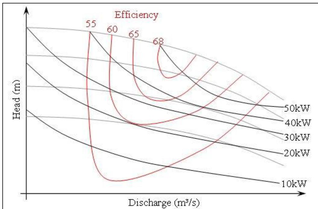
Figure 1 Sample of Pump Characteristic Curves
