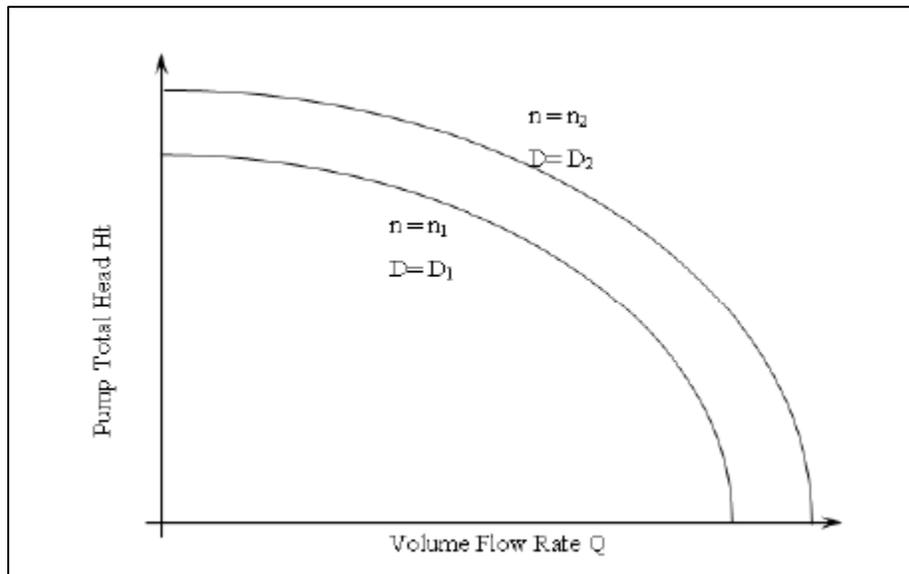
Figure 5 Relationship of performance characteristics for geometrically similar machines operating at different speeds
