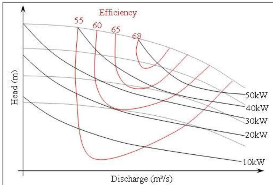
Figure 3 Family of Efficiency Curves overlain with other Characteristic Curves
