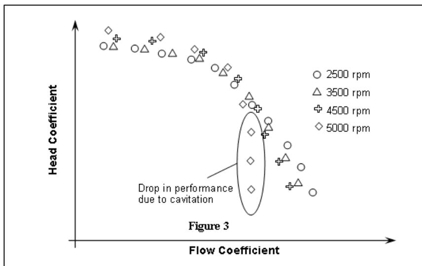
Figure 4 Dim-Less head - flow rate characteristics of a particular centrifugal pump operated at different speeds
