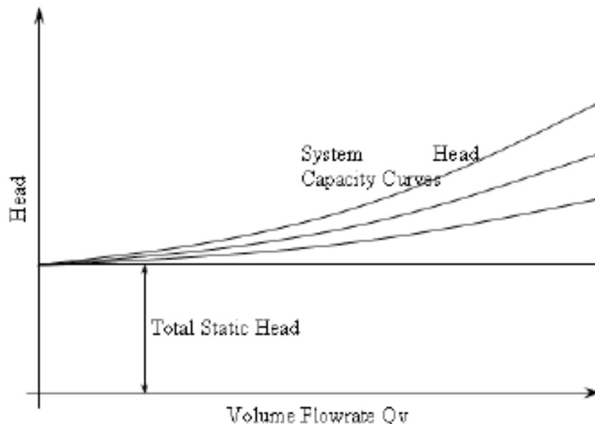
Figure E1: Typical head - flow curves for a pumping installation (pipes, valves etc.)
