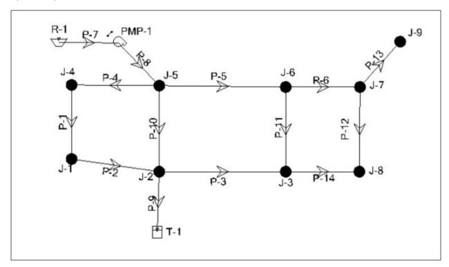
You are to determine the pipe diameters in the network to minimize the installation cost assuming all the pipes are ductile iron. Use the Darwin Designer to determine the total cost and size each pipe for each of the following conditions. Use the pipe cost information from Tutorial 4 the ductile iron pipe.
