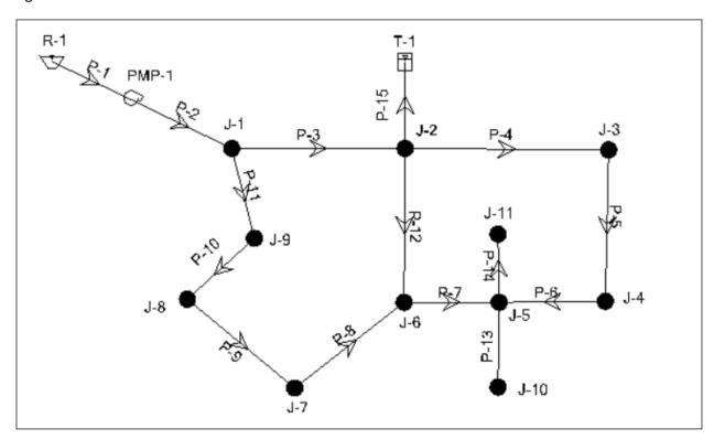
The source of water for the system is a pumped well. The water is treated and placed in a ground-level tank (shown above as a reservoir because of its plentiful supply), which is maintained at a water surface elevation of 210 ft. The water is then pumped from this tank into the rest of the system.
