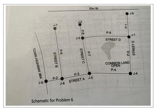
Currently, a model of the entire water system does not exist. However, hydrant tests were conducted hydrants located on two water mains, one in Town Highway #64 and the other on Elm Street. The following data were obtained:
